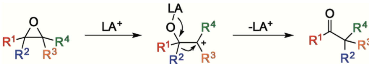
Fig. 1 Mechanism of the Meinwald rearrangement of epoxides activated by a Lewis acid.
